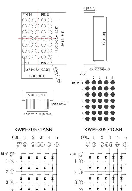
NOTES: All dimensions are in millimeters (inches) tolerance are  $\pm 0.25$ mm (0.01inch) unless otherwise noted.
