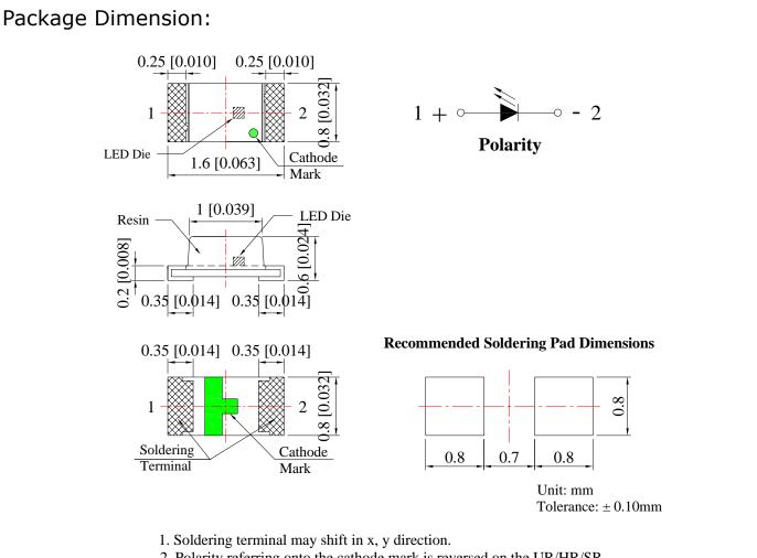
2. Polarity referring onto the cathode mark is reversed on the UR/HR/SR.
