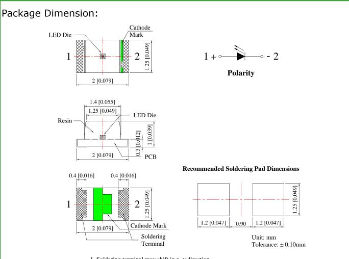
1. Soldering terminal may shift in x, y direction.
