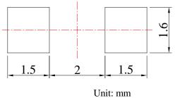
Tolerance:  $\pm 0.10 \text{ mm}$
