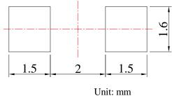
Tolerance:  $\pm 0.10 \text{ mm}$
