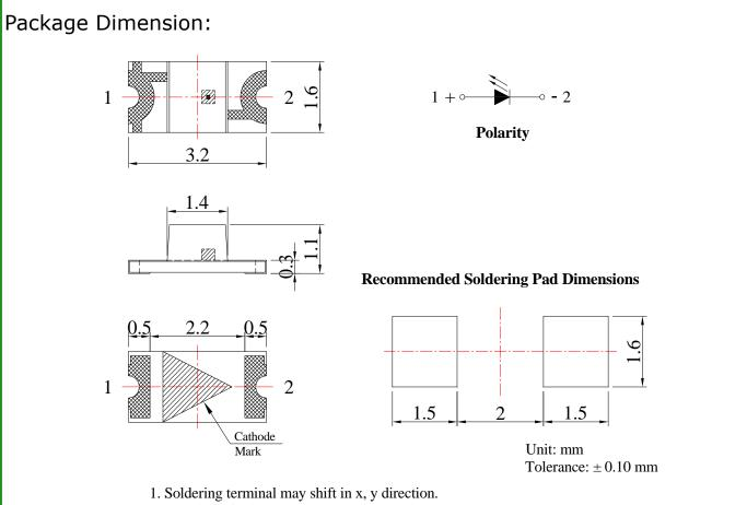
2. Polarity referring onto the cathode mark is reversed on the UR/HR/SR.
