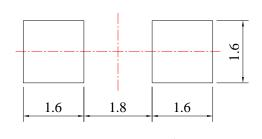
Unit: mm Tolerance: ± 0.10mm
