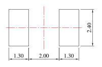
Unit: mm Tolerance: ± 0.10 mm
