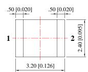
**Recommended Soldering Pad Dimensions**
