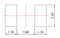
Unit: mm Tolerance: ± 0.10 mm
