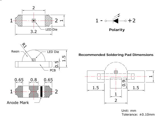
1. Soldering terminal may shift in x, y direction.
