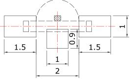
Unit: mm Tolerance:  $\pm 0.10$ mm
