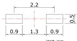
Unit: mm Tolerance: ±0.10mm
