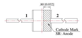
Unit: mm Tolerance: ± 0.10 mm
