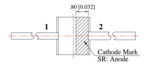
Unit: mm Tolerance: ± 0.10 mm
