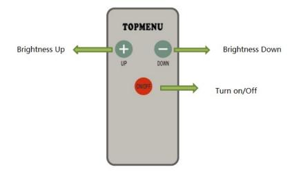
Notes: Only in AC status, the bulb can be controlled to turn on/off,dim brightness by Remote controller, and the brightness level is 10%,20%,30%,40%,50%,60%,70%,80%,90%,100%.
