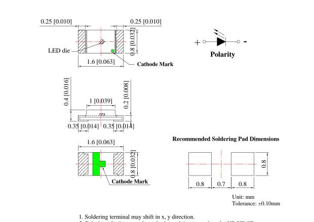
2. Polarity referring onto the cathode mark is reversed on the UR/HR/SR.
