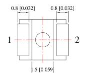
**Recommended Soldering Pad Dimensions**
