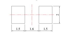
Unit: mm Tolerance: ± 0.10mm
