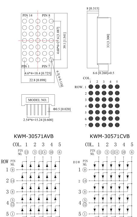
NOTES: All dimensions are in millimeters (inches) tolerance are  $\pm 0.25$ mm (0.01inch) unless otherwise noted.
